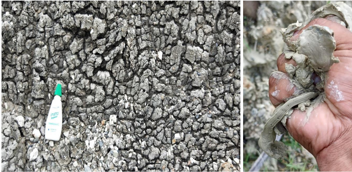
Figure 31. Cracking and plasticity test in field
