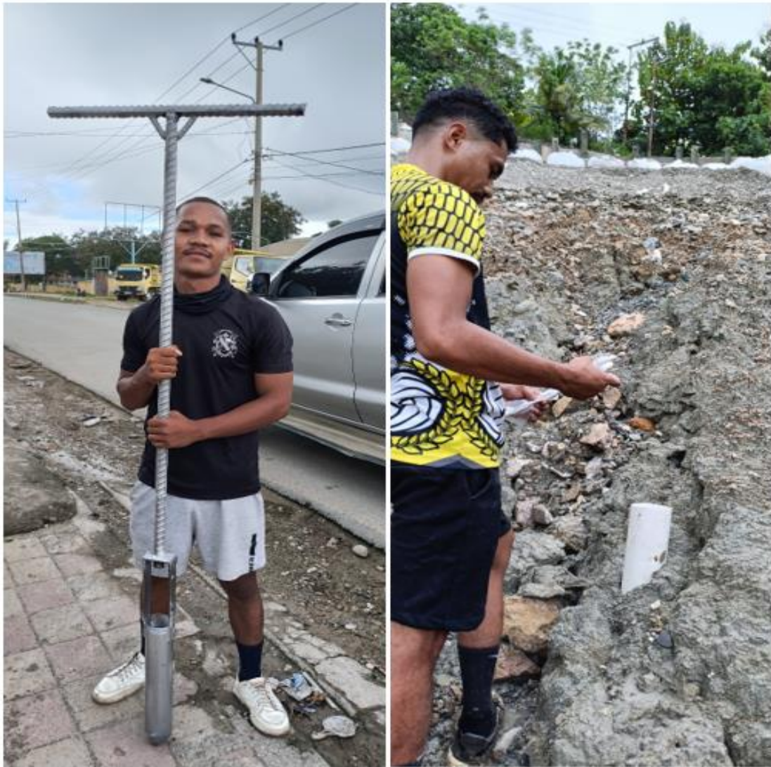
Figure 12. Hand auger (left), pipe tube for collecting the undisturbed sample
